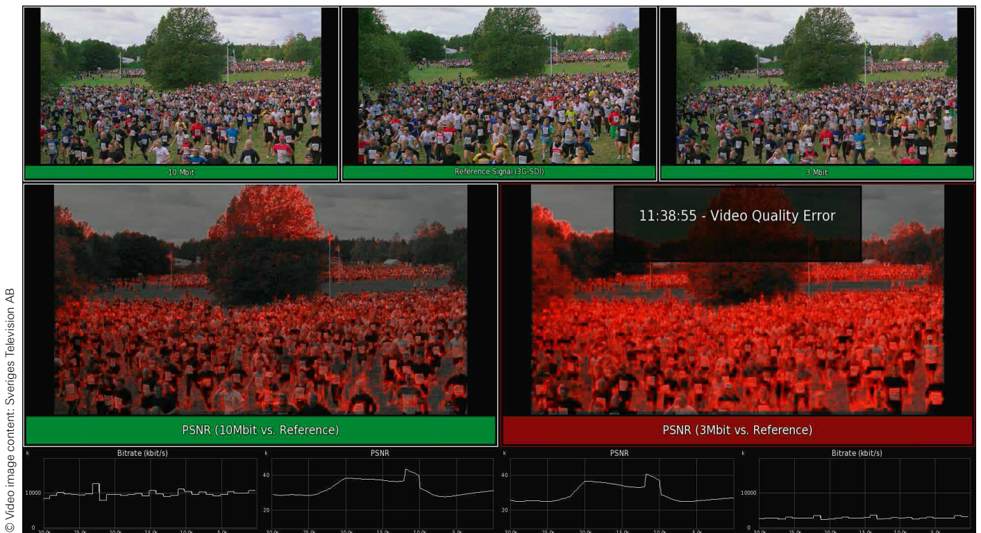
Fig. 6: Sample screenshot of a video live quality measurement with R&S®PRISMON.
