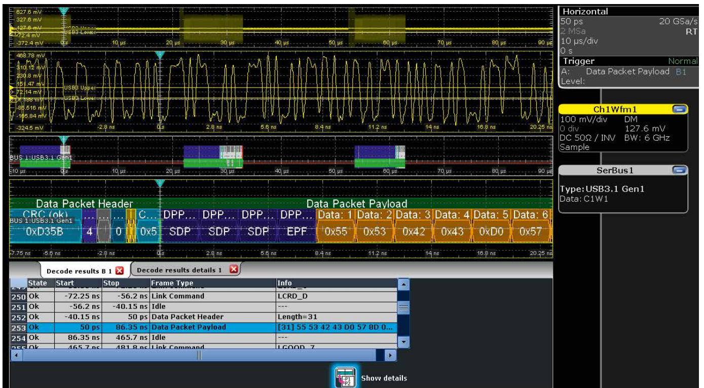
Fig. 13: Example of data decoding in line with USB 3.1 Gen 1.
