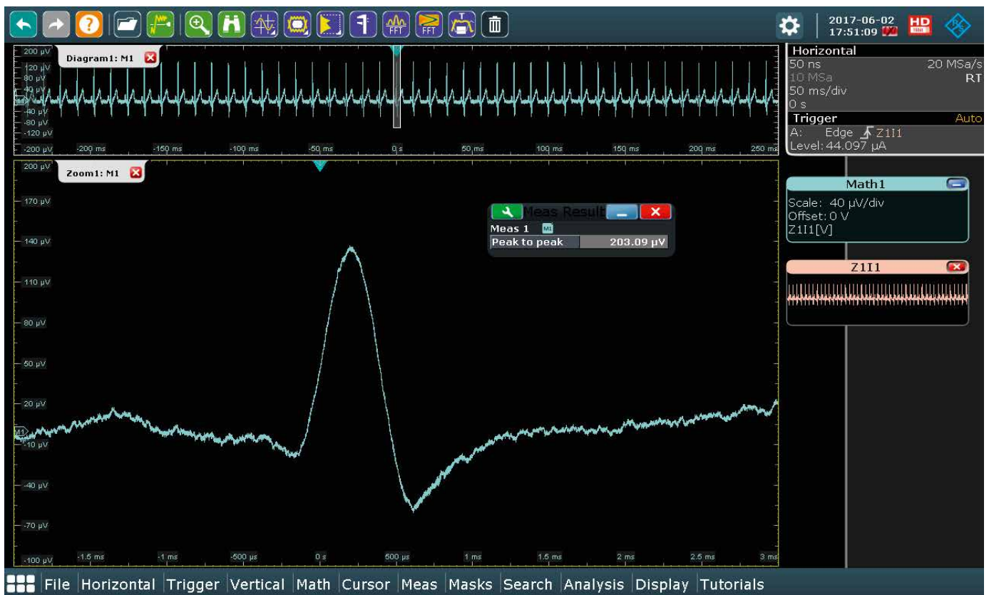
Fig. 6: Operating the probe with an external shunt turns the current measurement input into a highly sensitive voltmeter. As a result, even very small signals such as a 200 \mu\text{V} cardiac pulse can easily be measured.
